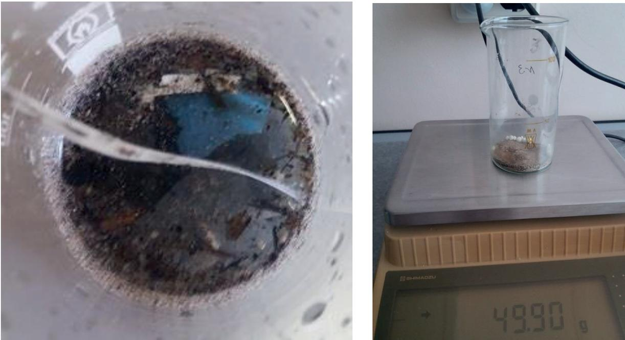
Fig.5. Left- a sample in a beaker before drying, right- a dried sample being weighed
