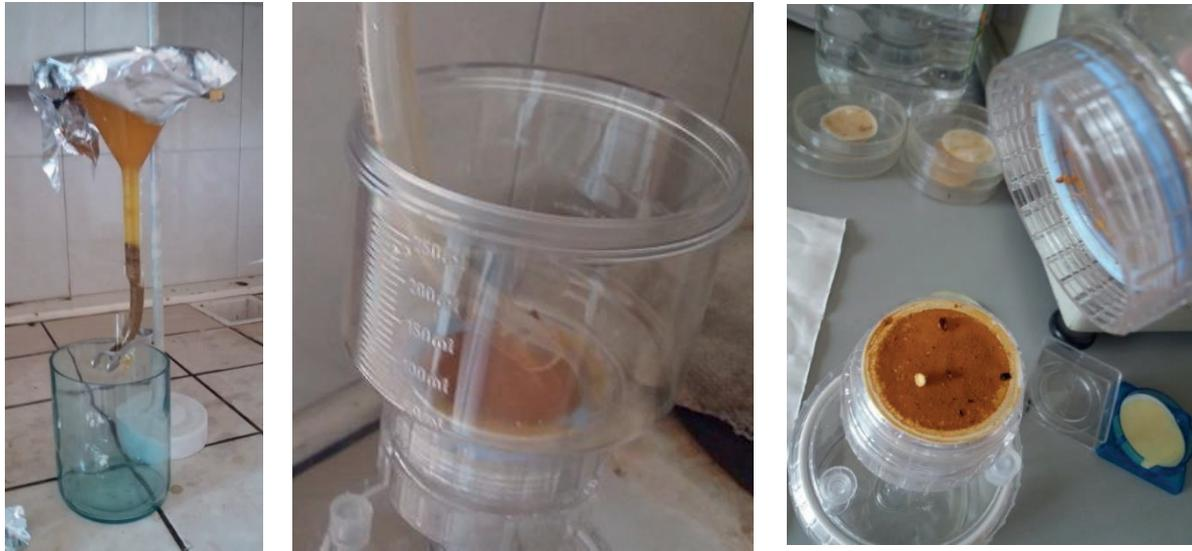
Fig.7. After density separation in a funnel, samples are transferred to polycarbonate filters.
