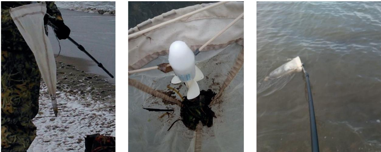
Fig. 2. Hand net sampling. Left to right – a) the net with a retractable rod, b) the flowmeter, c) sampling
